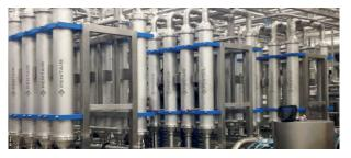
Four membrane units - Capacity to treat 6 ton/h of skimmed milk
