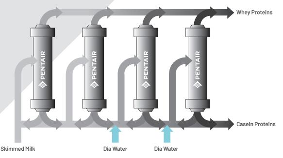
A membrane cascade system for separation of casein and whey proteins from skimmed milk
